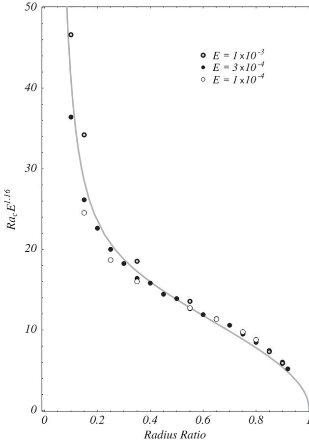
FIGURE 3 Modified critical Rayleigh number  $Ra_c E^{1.16}$  plotted as a function of radius ratio  $\chi$ . Points plotted are the same as in Fig. 2. Here, shaded circles, filled circles, and open circles represent results from numerical calculations with Ekman numbers  $E = 10^{-3}$ ,  $3 \times 10^{-4}$  and  $10^{-4}$ , respectively. The solid grey curve is produced using (9).
