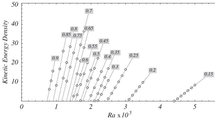
FIGURE 1 The fluid kinetic energy density, as a function of the Rayleigh number, calculated in spherical shells with different geometries. The graph corresponds to the  $E = 3 \times 10^{-4}$  calculations performed using 4-fold  $\phi$ -symmetry. The tag on each line shows the corresponding radius ratio.
